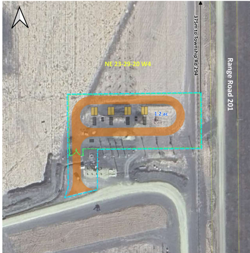
Figure 1. Location of new BESS equipment at the Michichi Solar Project. (The blue dashed line represents the total maximum construction area, the orange areas represent new roads for emergency vehicles to go around the batteries, the yellow rectangles show the battery container locations, and the black rectangles represent the inverters and electrical equipment.)
